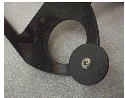
Figure 3 - Skid mounted ballast for fine-tuning balance
